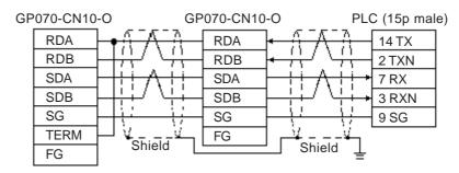
• When using Digital's Multi-link Cable, GP230-IS12-O
