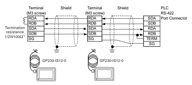
\*1 Please attach the termination resistor if needed. For the details, refer to the manual of the PLC.
