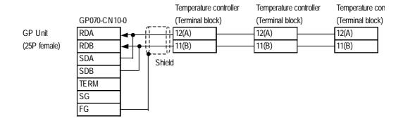
• When using Digital's RS-422 cable, GP230-IS12-O
