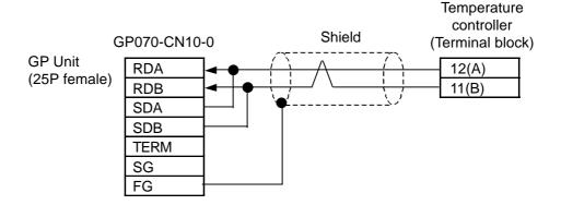
• When using Digital's RS-422 cable, GP230-IS12-O
