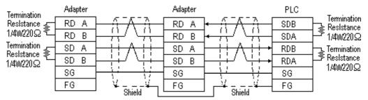
• When using Digital's Multi-link Cable, GP230-IS12-O
