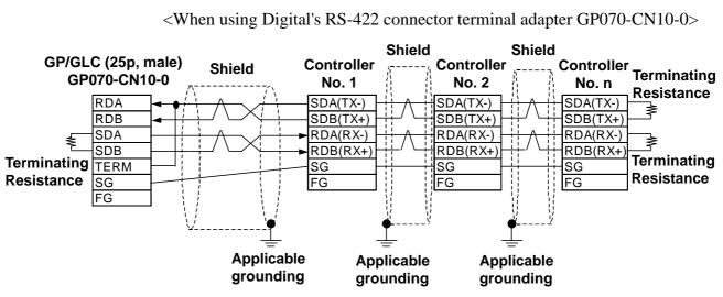
Cable Diagram 2 (1:n) (RS-422 4 Wires)
