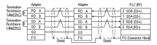
• When using Digital's Multi-link Cable, GP230-IS12-O
