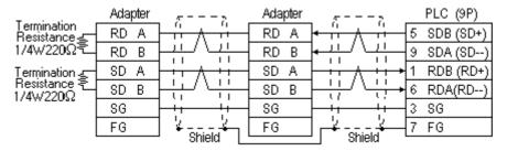
• When using Digital's Multi-link Cable, GP230-IS12-O
