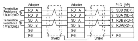
• When using Digital's Multi-link Cable, GP230-IS12-O
