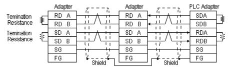
\* Check the PLC Adapter specifications for the Temination Resistance
