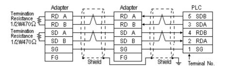
• When using Digital's Multi-link Cable, GP230-IS12-O
