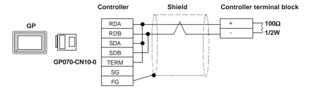
• Using Digital's RS-422 Cable GP230-IS11-0
