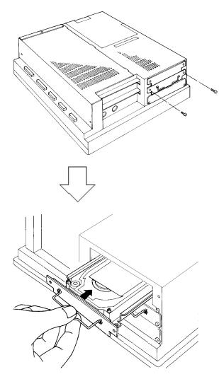
1) Unscrew the expansion slot's two (2) blank panel screws, and remove the blank panel.
