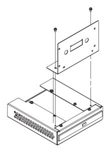
3) Secure the front face fastener to the PL-DK210 unit using the two (2) attachment screws.
