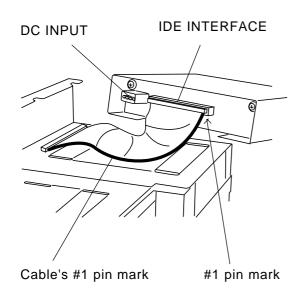
4) Connect the PL-DK210 unit to the PL unit via the connection cable. Be sure to confirm that the Cable's #1 pin mark and the connector are correctly aligned.
