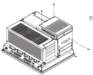
5) Secure the PL-DK210 unit to the PL unit using the four (4) attachment screws. Place the cable in the aperture between the PL-DK210 and PL units.
