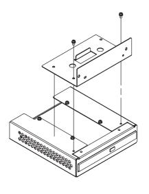
3) Secure the front face fastener to the PL-DK210 unit using the two (2) attachment screws.
