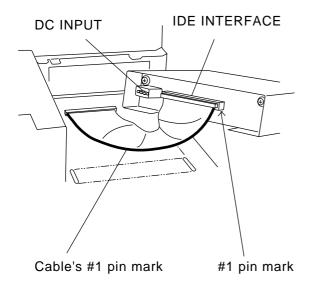
4) Connect the PL-DK210 unit to the PL unit via the connection cable.Be sure to confirm that the Cable's #1 pin mark and the connector are correctly aligned.
