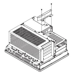
2) Secure the rear face fastener to the rear of the PL unit using the two (2) attachment screws.
