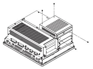
5) Secure the PL-DK210 unit to the PL unit using the four (4) attachment screws. Place the cable in the aperture between the PL-DK210 and PL units.
