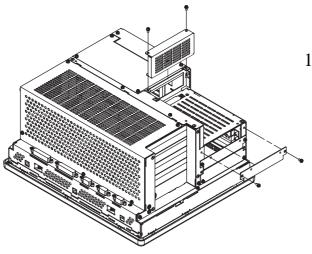
1) Unscrew the IDE I/F cover's two (2) attachment screws and the HDD1 slot's two (2) attachment screws. Remove the IDE I/F cover and the HDD1 slot cover.
