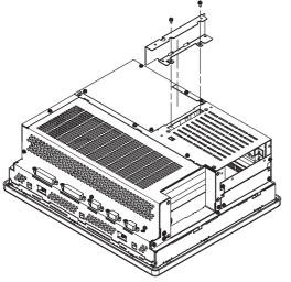
2) Secure the rear face fastener to the rear of the PL unit using the two(2) attachment screws.
