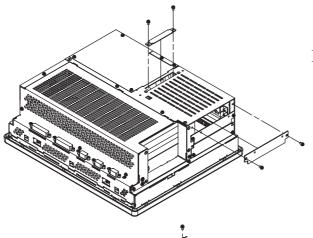
1) Unscrew the IDE I/F cover's two (2) attachment screws and the HDD1 slot's two (2) attachment screws. Remove the IDE I/F cover and the HDD1 slot cover.
