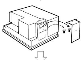
2) Remove the HDD cover and unscrew the HDD unit's two(2) set screws.
