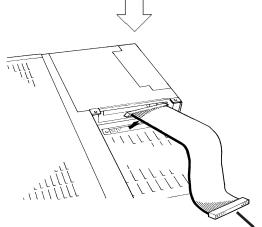
2) Connect the PL-DK200 to the PL unit via the connection cable PL-X900/PL-X920 series unit's.
