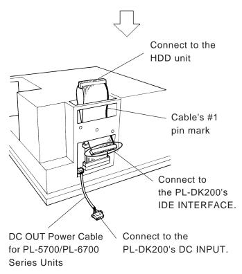
6) Connect the PL-DK200's DC OUT power cable for PL-5700/6700 Sereis Units (accessory) to the PL's DC OUT connector.
