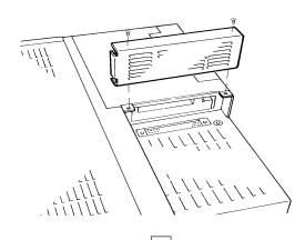
1) Unscrew the IDE I/F cover's two(2) attachment screws and remove the cover.
