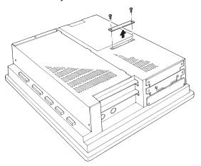
1) Unscrew the IDE I/F cover's two(2) attachment screws and remove the cover.
