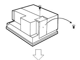
1) Remove the HDD unit protective cover's two(2) attachment screws.
