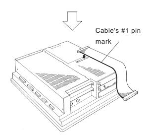
2) Connect the PL-DK200 to the PL unit via the connection cable PL-5900/PL-5910/PL-X900/PL-X920 series units.
