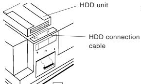
3) Disconnect the HDD unit from the HDD connection cable.
