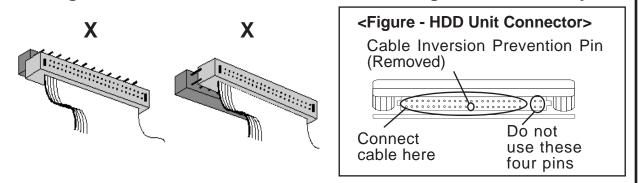
Also, be sure the hard disk unit cable's main board connector is not skewed from its correct attachment position (see above examples). Incorrect attachment can cause damage to the PL unit.
