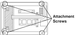
4) Unscrew the upper and lower backlight holder attachment screws, and remove the upper backlight unit's metal cover.
