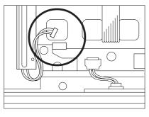
3) Disconnect the upper backlight's power connector.
