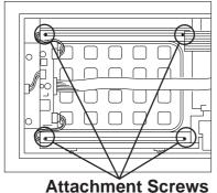
4) Loosen the upper and lower backlight holder attachment screws, and remove the upper backlight unit's metal cover.
