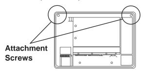
1) Turn the GP's power OFF (i.e. disconnect the GP's power cord). Use a Phillips screwdriver to remove the case's two (2) rear attachment screws, and pivot the rear cover open, starting from the top of the unit.
