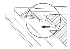
3) Disconnect the upper backlight's power connector.
