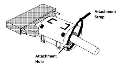
2) Confirm that the Ferrite Core is held close to the connector cover, as shown below, and then tighten the attachment strap. Any remaining strap material should be cut off.
