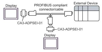
**NOTE** • The cable length must be 50m or less in one segment.
