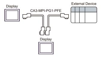
**NOTE** • The cable length must be 50m or less in one segment.
