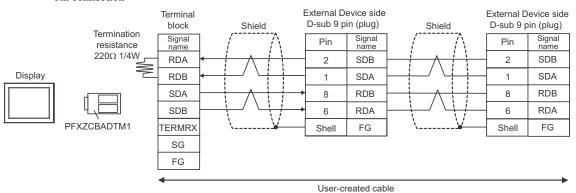
• The cable length must be 500m or less.
