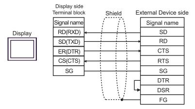
• When the External Device supports DTR/DSR control
