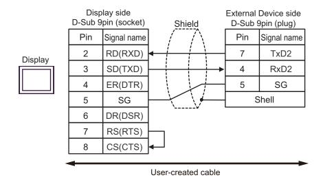
Only the COM port which can communicate by RS-232C can be used. "■ IPC COM Port" (page 5) \*2
