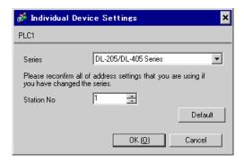
For communication settings, use the DIP switches on the CPU unit. To set the station No., use the instruction word programmer (S-01P). After completing the settings, reboot the External Device to enable them. Please refer to the manual of the External Device for details.
