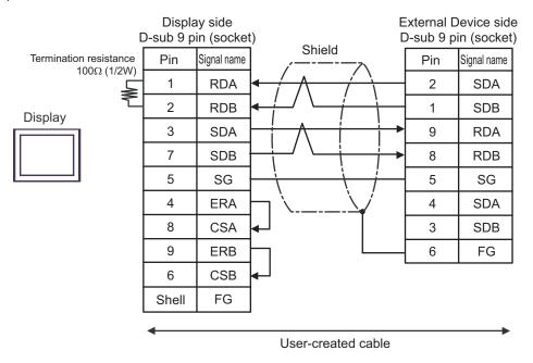
\* Termination resistance switch on the communication module should be set "3".
