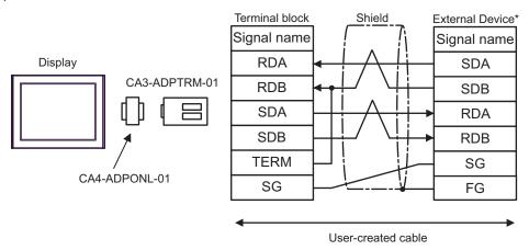
\* Turn On the termination resistance switch of the External Device, and set the operation mode to 3. 5F)
