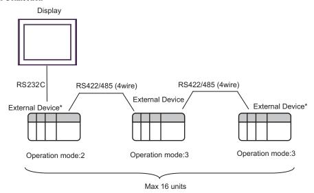
\* Turn ON the termination resistance switch on the interface which terminates the RS422 connection.
