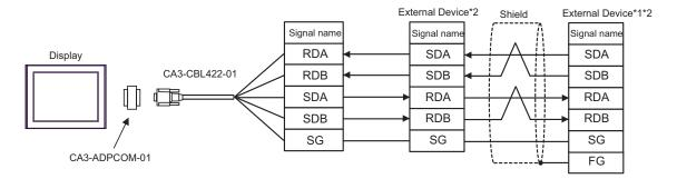
Do not connect the FG terminal of CA3-CBL422-01 to the External Device.
