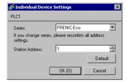
To configure communication settings, use the FUNC/DATA, Up, Down, or PRG/RESET key on the touch panel located on the front of the External Device. Refer to your External Device manual for details.
