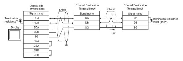
\*1 Use a built-in resistance in the Display as termination resistance. Set the DIP Switch on the rear side of the Display as below.
