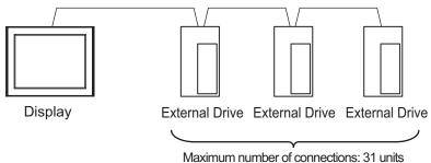
• Using 1 port (when connecting External Devices)
