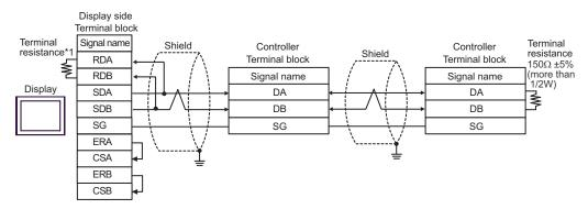
\*1 The resistance in the Display is used as the termination resistance. Set the value of the DIP Switch on the rear of the Display as shown in the table below.
