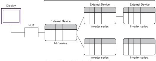
Between Display and MP series: Ethernet connection Between MP series and Inverter series: MECHATROLINK connection Between Inverter series and Inverter series: MECHATROLINK connection
