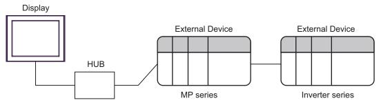
Between Display and MP series: Ethernet connection Between MP series and Inverter series: MECHATROLINK connection
