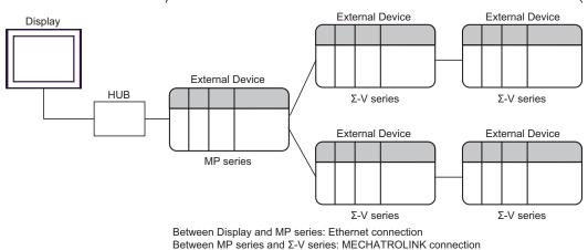
Between MP series and  $\Sigma$ -V series: MECHATROLINK conne  $\Sigma$ -V series and  $\Sigma$ -V series: MECHATROLINK connection
