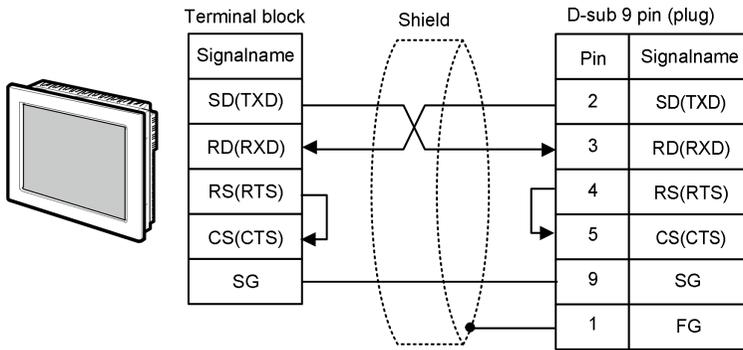
**NOTE** • The cable length must be 15m or less.
