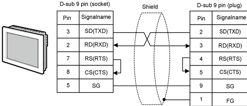
**NOTE** • The cable length must be 15m or less.
