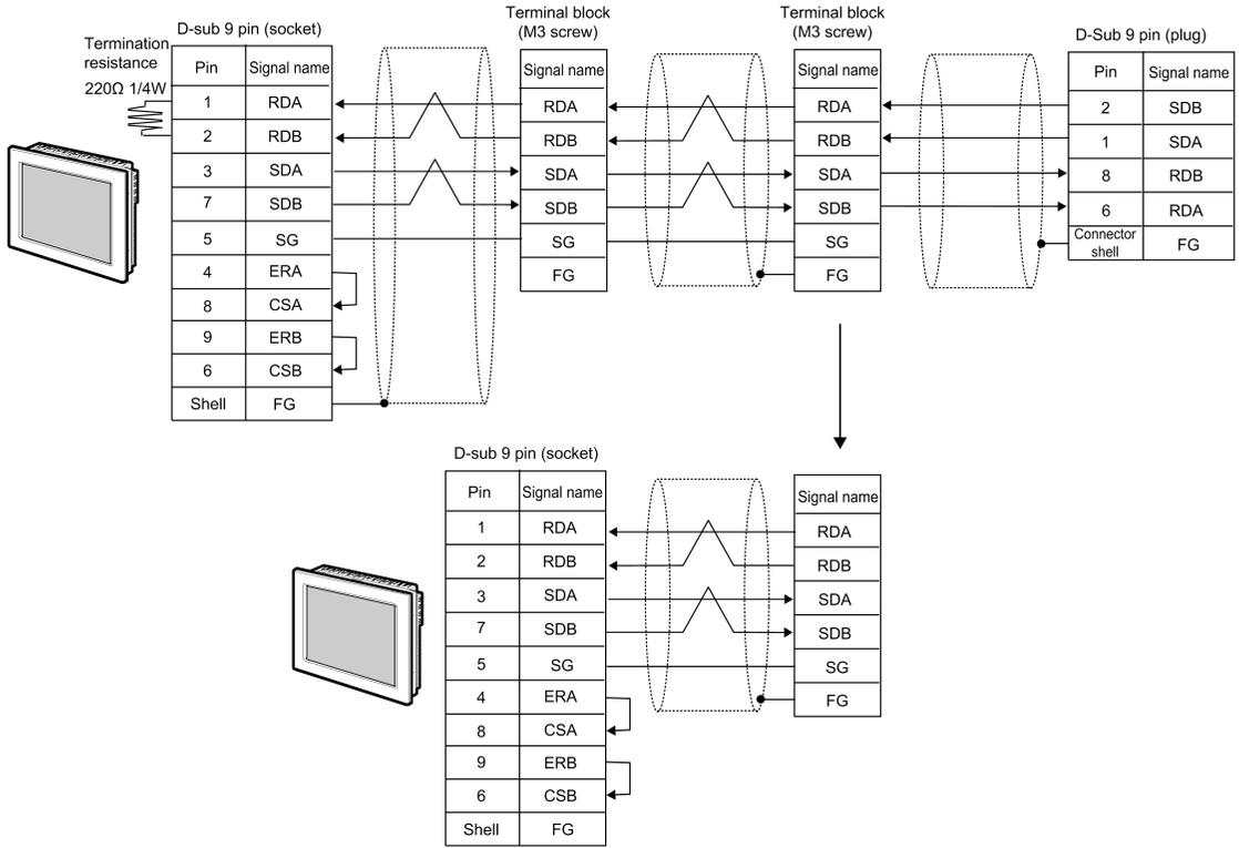
**NOTE** • The cable length must be 500m or less.
