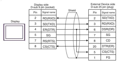
1C) Display side External Device side Terminal block D-sub 25 pin (plug) Shield Signal name Pin Signal name RD(RXD) 2 SD(TXD) Display 3 RD(RXD) SD(TXD) 6 DSR(DR) ER(DTR) 7 SG SG 8 CD RS(RTS) 20 DTR(ER) CS(CTS) 5 CS(CTS)
