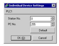
Use the DIP switch of the Computer Link Unit for setting. Please refer to the manual of the External Device for more details.
