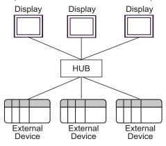
\* The maximum number of connectable units varies depending on the External Device. Refer to your External Device manual for details.
