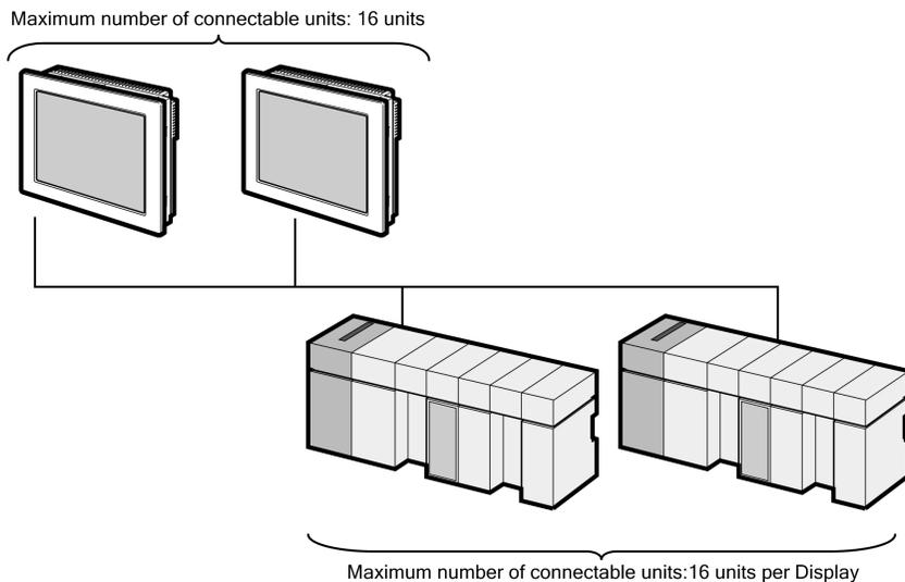
**NOTE** • The maximum number of connectable Displays is 16 units. However, keeping performance in consideration, the number of Displays that can be substantially used is up to 4.
