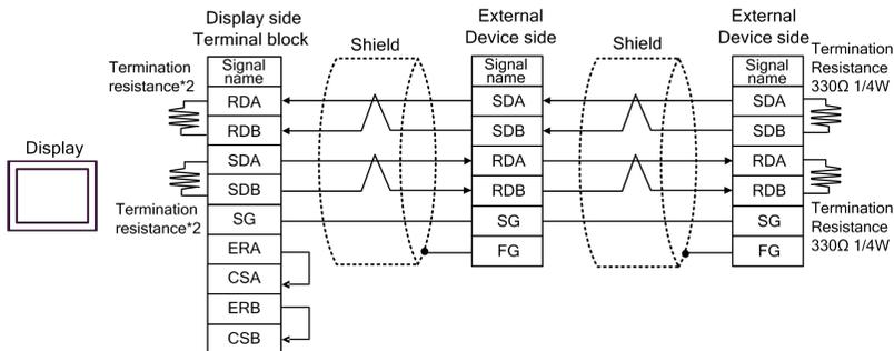
\*2 The resistance in the Display is used as the termination resistance. Set the value of the DIP Switch on the rear of the Display as shown in the table below.
