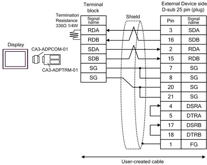
**NOTE** • As the External Device has the termination resistance built-in, you do not need to connect the termination resistance.
