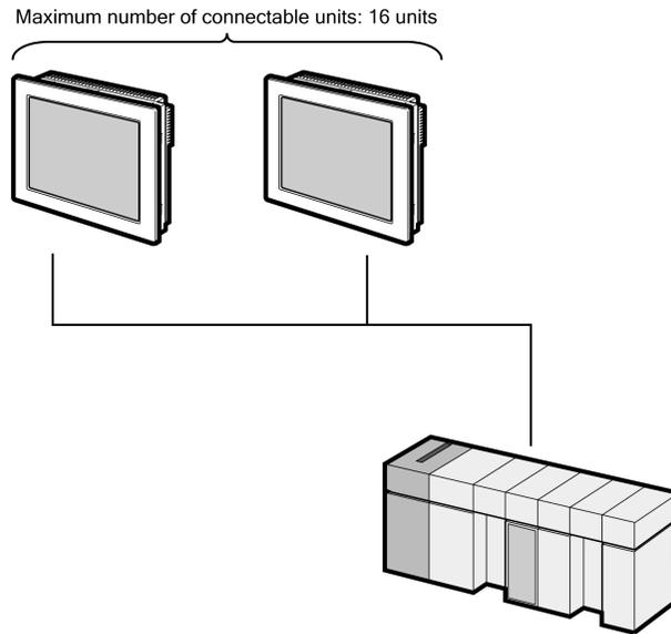
**NOTE** • The maximum number of connectable Displays is 16 units. However, keeping performance in consideration, the number of Displays that can be substantially used is up to 4.
