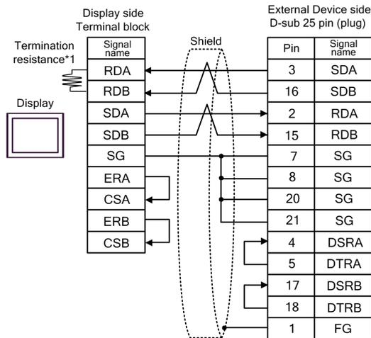
**NOTE** • As the External Device has the termination resistance built-in, you do not need to connect the termination resistance.
