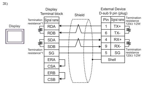
\*1 The resistance in the Display is used as the termination resistance. Set the value of the DIP Switch on the rear of the Display as shown in the table below.
