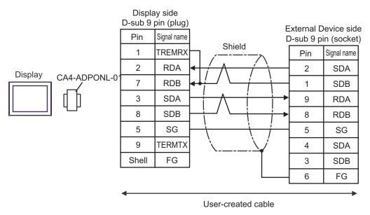
\* Termination resistance switch on the communication module should be set "3".
