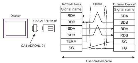
\* Turn On the termination resistance switch of the External Device, and set the operation mode to 3.
