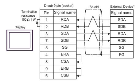
\* Turn On the termination resistance switch of the External Device, and set the operation mode to 3.
