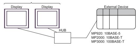
\*2 When Ethernet port on CPU unit in MP2310/MP2300S/MP2400 is used, up to 4 Displays can be connected.
