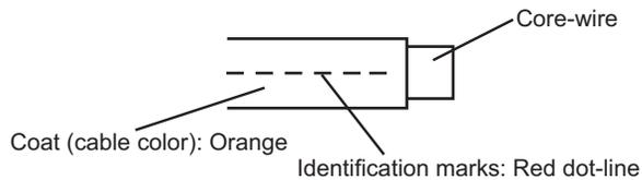
In the example above, the cable color is orange, and the identification mark shows red dot-line, which means TXD.
