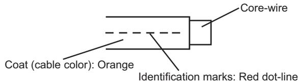
In the example above, the cable color is orange, and the identification mark shows red dot-line, which means TXD.
