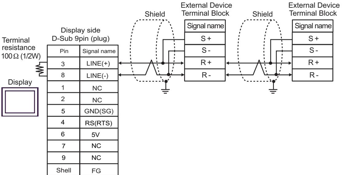
**IMPORTANT** • The 5V output (Pin #6) on the Display is the power for the Siemens AG's PROFIBUS connector. Do not use it for other devices.
