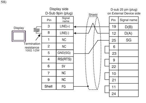
• The 5V output (Pin #6) on the Display is the power for the Siemens AG's PROFIBUS connector. Do not use it for other devices.
