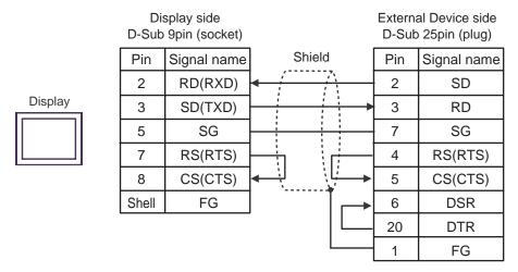
1B) External Device side Display side Terminal Block D-Sub 25pin (plug) Shield Pin Signal name Signal name RD(RXD) 2 SD Display SD(TXD) 3 RD SG 7 SG RS(RTS) 4 RS(RTS) CS(CTS) 5 CS(CTS) 6 **DSR** 20 **DTR** 1 FG
