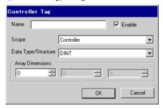
5) Input the Controller Tag Name, Scope, Data Type/Structure, and Array Dimensions. To use a created tag, select [Enable] and then click [OK].
