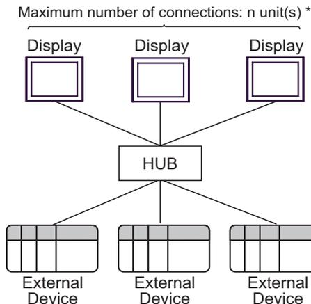
\* The maximum number of connectable units varies depending on the External Device. Refer to your External Device manual for details.
