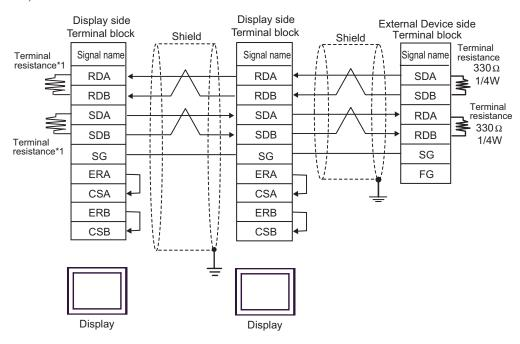
\*1 The resistance in the Display is used as the termination resistance. Set the value of the DIP Switch on the rear of the Display as shown in the table below.
