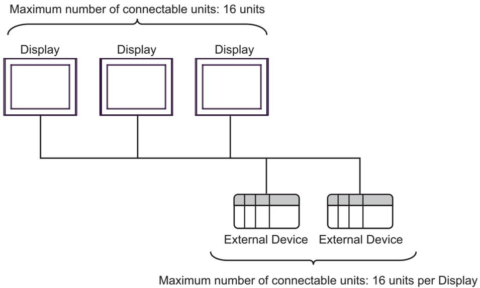
**NOTE** • The maximum number of connectable Displays is 16 units. However, keeping performance in consideration, the number of Displays that can be substantially used is up to 4.
