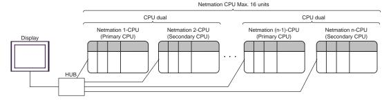
• 1:n Connection (Ethernet single/Netmation CPU single/dual mixed)
