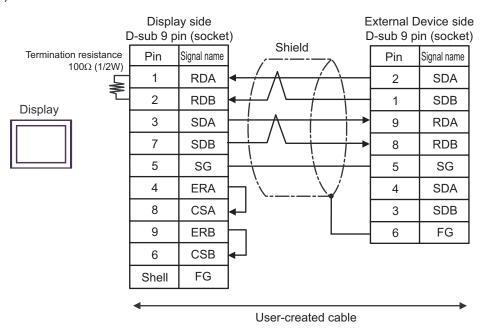
\* Termination resistance switch on the communication module should be set "3".
