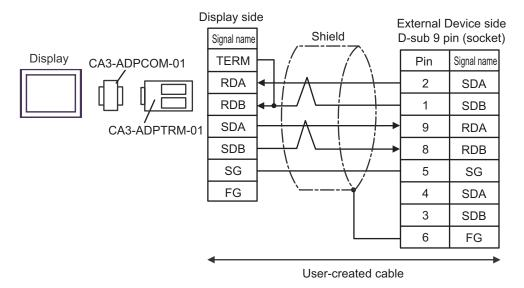
\* Termination resistance switch on the communication module should be set "3".
