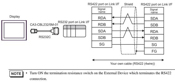
• For the 1st External Device connected with RS232C and RS422, set the operation mode on the Link I/F to 2. For the following External Devices connected with RS422, set it to 3.
