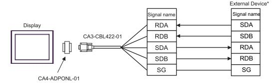
Do not connect the FG terminal of CA3-CBL422-01 to the External Device.
