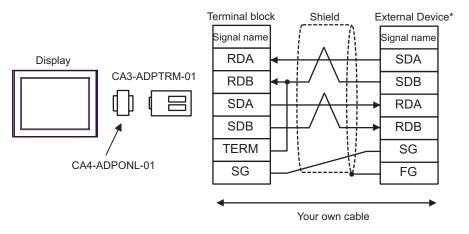
\* Turn On the termination resistance switch of the External Device, and set the operation mode to 3.
