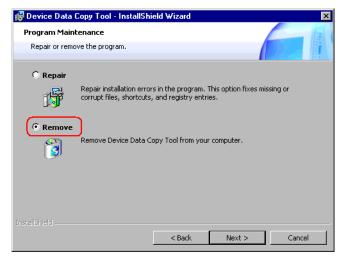
5 Click [Remove] to uninstall the Device Data Copy Tool.
