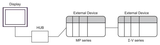
Between Display and MP series: Ethernet connection Between MP series and  $\Sigma$ -V series: MECHATROLINK connection
