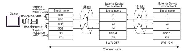
• When IPC is used as the Display, the terminal resistance of  $220\Omega$  can be inserted by the fact that the dip switch 5, 6 of IPC is turned to ON.
