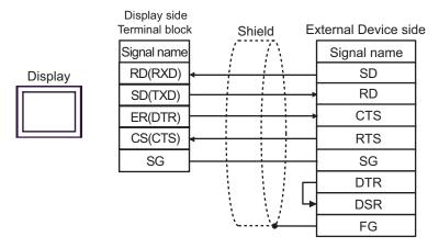
• When the External Device supports DTR/DSR control
