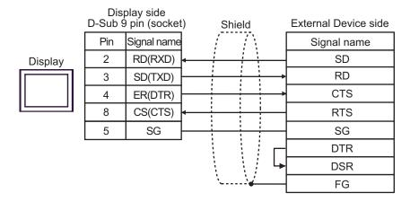
• When the External Device supports DTR/DSR control
