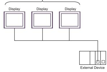
**NOTE** • The maximum number of connectable Displays is 16 units. However, keeping performance in consideration, the number of Displays that can be substantially used is up to 4.
