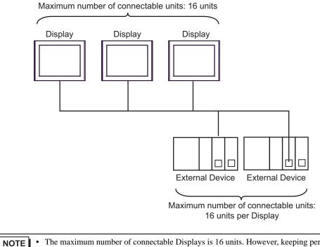
• The maximum number of connectable Displays is 16 units. However, keeping performance in consideration, the number of Displays that can be substantially used is up to 4.
