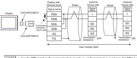
• Use the DIP switch in the communication cassette to set the termination resistance. Set SW1-1 of the External Device which terminates the connection to ON.
