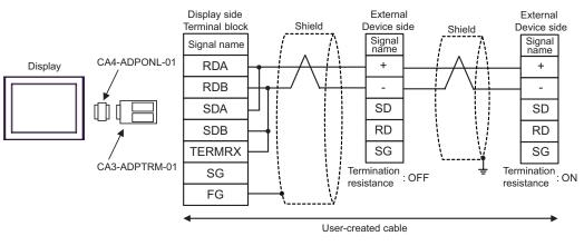
**NOTE** • Use the DIP switch in the communication cassette to set the termination resistance. Set SW1-1 of the External Device which terminates the connection to ON.
