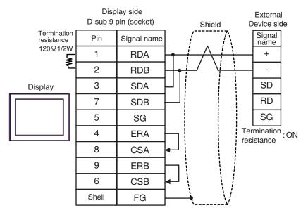
**NOTE** • Use the DIP switch in the communication cassette to set the termination resistance. Set SW1-1 of the External Device to ON.
