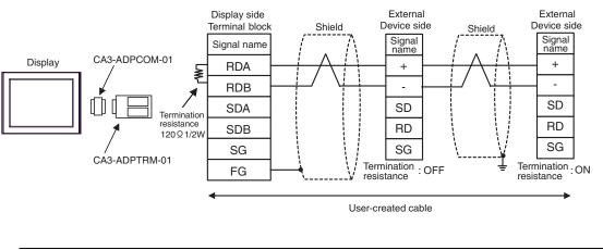
• Use the DIP switch in the communication cassette to set the termination resistance. Set SW1-1 of the External Device which terminates the connection to ON.
