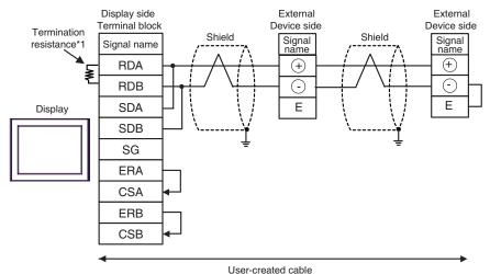
IMPORTANT • Use the lead wire to connect between "-" terminal and "E" terminal in the External Device which terminates the connection.
