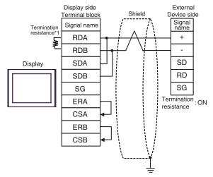
• Use the DIP switch in the communication cassette to set the termination resistance. Set SW1-1 of the External Device to ON.
