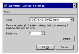
Use the ladder software (DirectSOFT32 programming version 4.0) for communication settings. After completing the settings, reboot the External Device to enable them. Please refer to the manual of the External Device for details.
