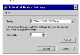
For communication settings, use the instruction word programmer (S-01P). After completing the settings, reboot the External Device to enable them. Please refer to the manual of the External Device for details.
