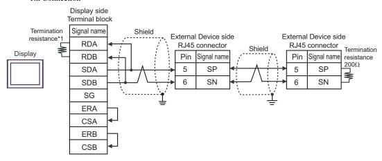
\*1 The resistance in the Display is used as the termination resistance. Set the value of the DIP Switch on the rear of the Display as shown in the table below.
