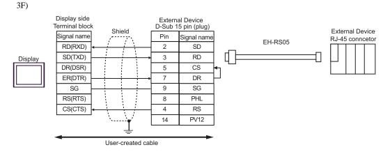
Display side External Device Terminal block D-Sub 15 pin (plug) External Device Shield RJ-45 conncetor Signal name Pin Signal name EH-RS05 RD(RXD) 2 SD RD SD(TXD) 3 Display DR(DSR) 5 CS ER(DTR) 7 DR 9 SG SG RS(RTS) 8 PHL CS(CTS) 4 RS 14 PV12 User-created cable
