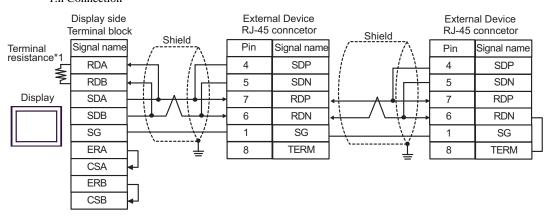
\*1 The resistance in the Display is used as the termination resistance. Set the value of the DIP Switch on the rear of the Display as shown in the table below.
