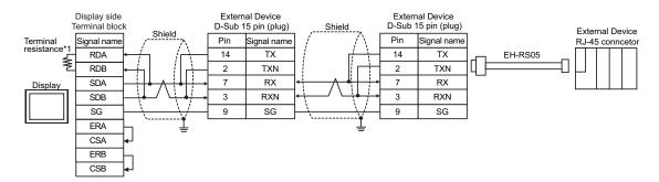
\*1 The resistance in the Display is used as the termination resistance. Set the value of the DIP Switch on the rear of the Display as shown in the table below.
